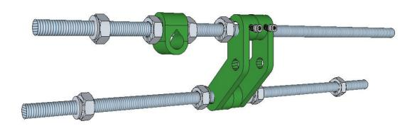
The right hand side is simply a repeat of the left. From left to right, the rod should have: 1 washer, 2 nuts, 1 washer, 1 bar clamp (slipped on to the rod), 1 washer, 2 nuts, and 1 washer.
